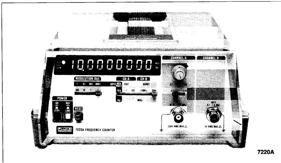
accuracy. There are two oven options to choose from, one with an accuracy of  $\pm 1 \times 10^7$ , and one with an accuracy of  $\pm 3 \times 10^8$  over the  $0^\circ\text{C}$  to  $40^\circ\text{C}$  temperature range.
